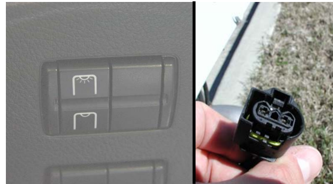
CODE L72 Instrument panel switch and wiring on rear cross-member. The interface supports bulb loads up to a maximum of 4 amps and ohmic loads up to a maximum of 10 amps.
