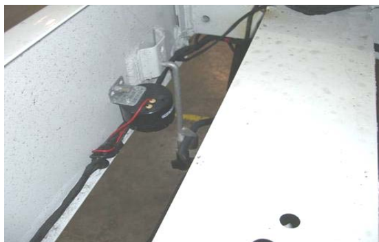
CODE JW0 alarm-rear backup, located at rear cross member
