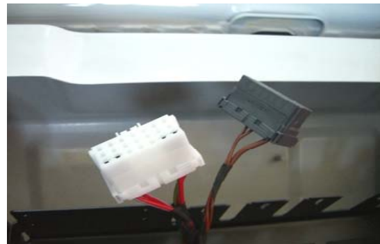
CODE ED8 PSM pre-wire, located in driver seat pedestal
